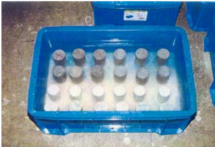
Photograph-3 Soaking test in a 5% sulfuric acid solution Cylinder type sample ( \text{Ø}5 \times 10 \text{ cm} )
