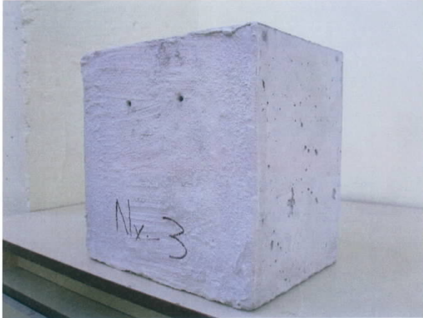
Fig. 1 – Test specimen of C 25/30 concrete with Xypex Concentrate crystallisation coat applied
