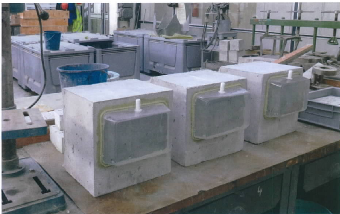
Fig. 2 – Test set - specimen with fixed container for simulation of loading by moisture
