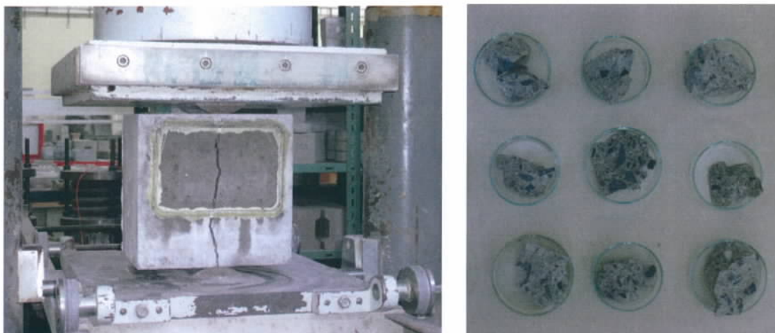
Fig. 5 – Breaking of the test specimen and samples taken for the gravimetric method
